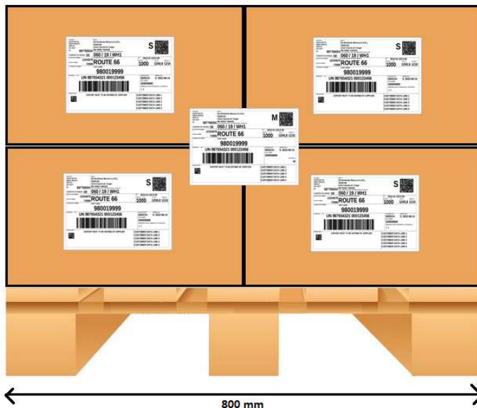
Figure 7: Example usage of the master label on an homogeneous pallet (1200X800mm) with A5 label format.
