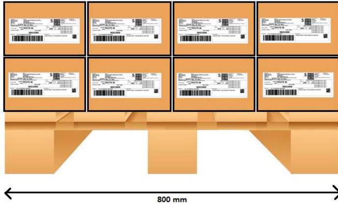
Figure 8: Example usage of single labels on an homogeneous pallet (1200X800mm) with SLC1 label format.
